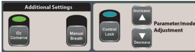
**O<sub>2</sub> Conserve** is used when an oxygen concentrator is employed as the oxygen source, or when the user wishes to conserve the remaining oxygen in a depleting cylinder. This function limits the amount of oxygen used during inspiration (either through the hose connector or the barbed tree connector) to 10 LPM. See **USING THE CCV WITH A CONCENTRATOR OR FLOWMETER** for more information.
