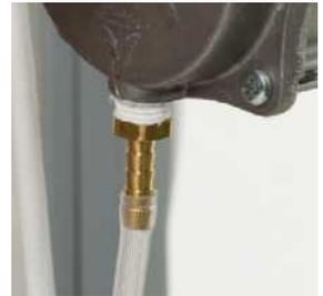
**NOTE:** In order to use the reservoir barb, the provided oxygen hose must be connected between the reservoir outlet and the CCV's DISS port. See **USING THE CCV WITH A CONCENTRATOR OR FLOWMETER** for more information.
