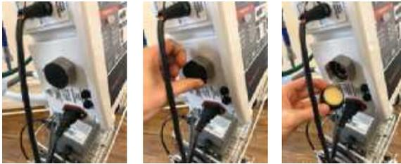
To replace the filter, remove the protective screen by prying it off with fingernails or a dull flat tool. Discard the filter, insert a fresh one, and replace the protective screen.
