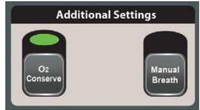
To enable O<sub>2</sub> Conserve mode, connect an oxygen source and ensure that Control Lock is not engaged. Press the O<sub>2</sub> Conserve button in the Additional Settings panel of the CCV interface. The green light will come on when O<sub>2</sub> Conserve mode is engaged.
